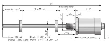
$^\star = 55$  mm up to stroke 1000 mm, from 1250 mm consider 60 mm due to M4 threaded hole
