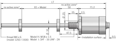
$^{*}$  = 55 mm up to stroke 1000 mm, from 1250 mm consider 60 mm due to M4 threaded hole
