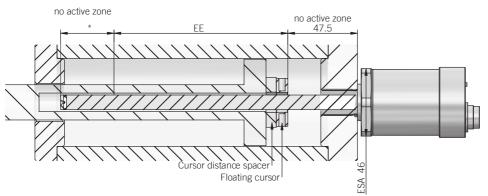
$^{\ast}$  = 55 mm up to stroke 1000 mm, from 1250 mm consider 60 mm due to M4 threaded hole
