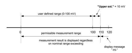
Fig. 6.3. Definition of measurement ranges (**mV** input)
