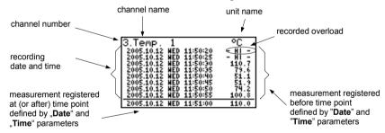
Fig. 6.16. Unit in "Measurements list" measurement results presentation mode. "List type" parameter set as "historic".
