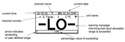
Fig. 6.14. Exceeding allowable range in "Single channel" mode
