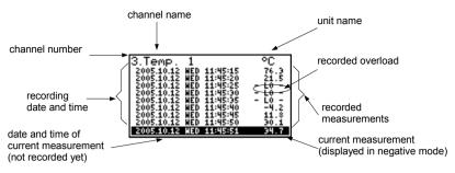
Fig. 6.15. Unit in "Measurements list" measurement results presentation mode.
