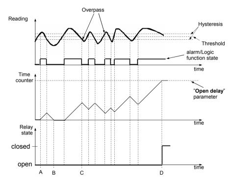
Fig. 6.31. Working output controlled by single channel alarm with large reading oscillations.
