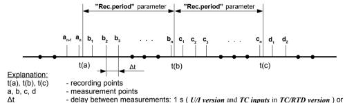
Fig. 6.6. Principle of measurement recording
