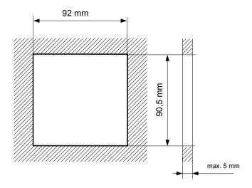
Fig. 4.2. Allowable mounting hole dimensions
