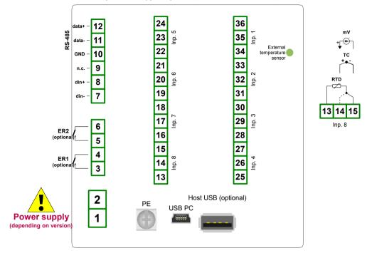
Fig. 4.14. Terminals description ( mV/RTD/TC version )
