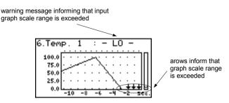
Fig. 6.20. Exceeding lower limit of the graph scale range
