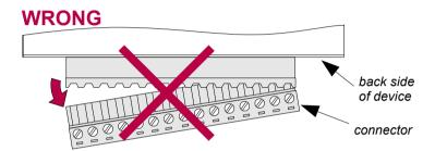
Fig. 4.4. Connectors removing method
