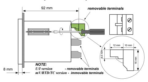
Fig. 4.3. Installing of brackets, and dimensions of connectors.
