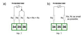
Fig. 4.16. Connection of Pt100 sensors for channel no 1:
