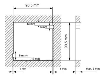
Fig. 4.1. Recommended mounting hole dimensions
