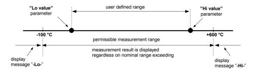
Fig. 6.4. Definition of measurement ranges (RTD input)
