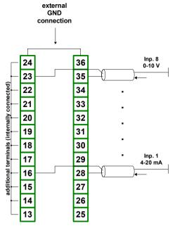
Fig. 4.12. Connections of current signals of active sensors (current signal 0-20 mA or 4-20 mA and ground)
