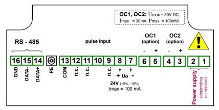
Figure 4.5. Terminals description (OC-type outputs)
