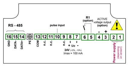
Figure 4.8. Terminals description (relay and active voltage outputs)
