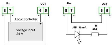
Figure 4.15. Example of OC-type outputs connection
