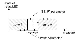
Figure 6.2. One threshold control of the relay/LED outputs
