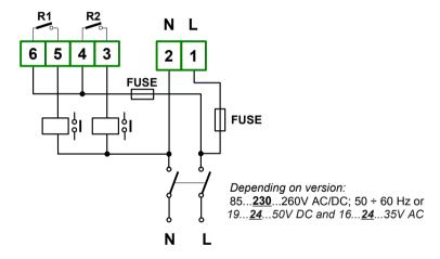
Figure 4.12. Connection of power supply and relays
