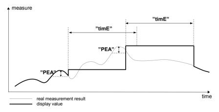
Figure 6.1. Process of peaks detection
