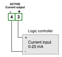
Figure 4.16. Example of active current outputs connection (for device with active current output only)
