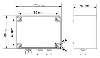
Figure 4.1. Device and assembly dimensions
