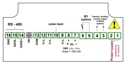
Figure 4.7. Terminals description (relay and passive current outputs)
