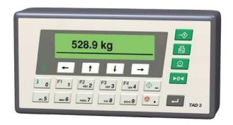
The batching version of the TAD 3 makes it possible to perform batching of up to six components in coarse and fine feeding phases. Other process functions like stirring, heating, dumping, etc. also can be controlled with the batching version.
