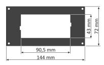
SMP-147/94 to mount 96 x 48 mm size unit in place of 144 x 72 mm cut-out
