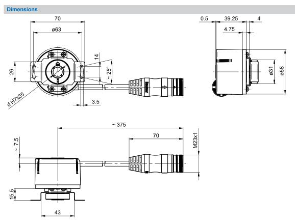
Through hollow shaft, flylead connector M23
