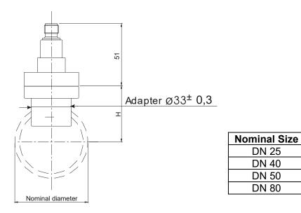
Position and weld-in the mounting adapter according to the nominal diameter suitable marking. The marking on the adapter must be in line with the outer diameter of the pipe. Also pay attention to the later position of the rotating vane (shaft of the vane shifted by 90° to the direction of flow).
