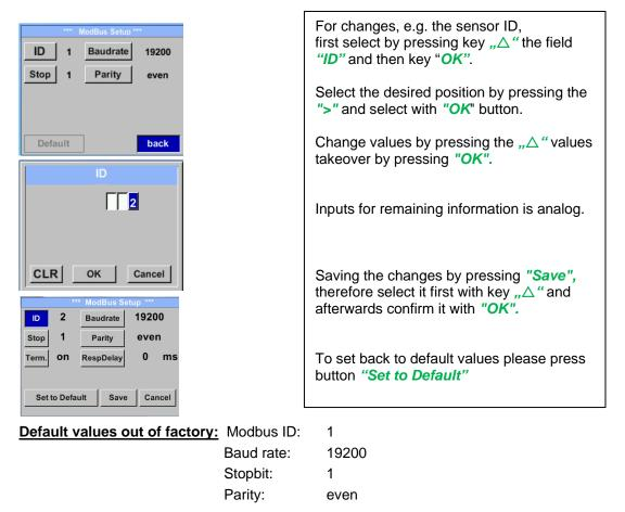
**Remark**: If the sensor placed at the end of the Modbus system a termination is required. Therefore, the enclosed 120R resistor is to be connected at Pin 1 and Pin 3 of connector "X2"
