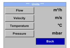
To make changes to the unit for the respective measurement value, first select by pressing " $\Delta$ " the field of the "measurement value" and activate "it with "*OK*".
