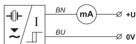
Fig. 28: Connection diagram of the ULS sensor with S type output (two-state current switch 4 mA / 20 mA)
