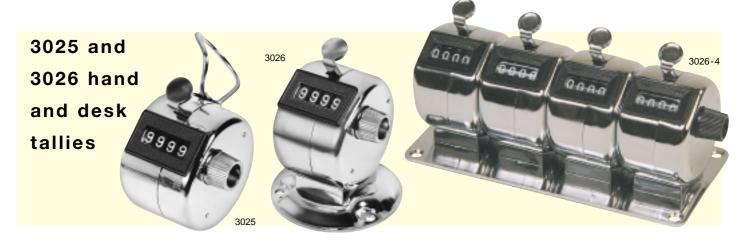
The count on both the Hand and Desk Tally is incremented by pressing the easy-action thumb button on the top of the unit. Reset to zero is by use of the side mounted knob. The Desk Tally is simply a bench mounted version of the Hand Tally and is supplied with an integral pre-drilled mounting plate.
