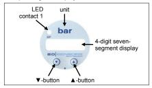
The device has, according to the order max, one LED which is allocated to the contact. The LED will light up when the set point has been reached and the contact is active. The display of the measured value as well as the configuration of the individual parameters occurs menu-driven via the sevensegment display
