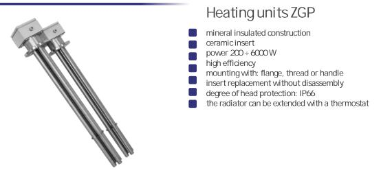
Heating units ZGP consist of tubular elements welded or brazed into a threaded screwplug which can then be inserted into a threaded opening in a tank wall or through a mating full or half coupling. Degree of head protection is IP66. Connection terminals and protective clamp are located under head cover. In the cover there is a gland through which the power cable is inserted.
