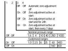
The switches 1 and 2 don't have any function at special pressure ranges.
