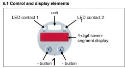
Fig. 2 touch pad (example with two contacts)
