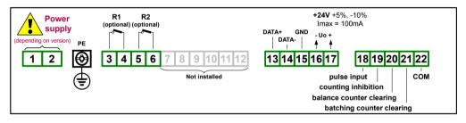
Figure 4.3. Terminals description (two relay outputs)
