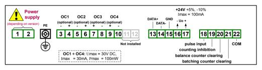
Figure 4.10. Terminals description (four OC-type outputs)
