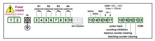
Figure 4.9. Terminals description (four relay outputs)
