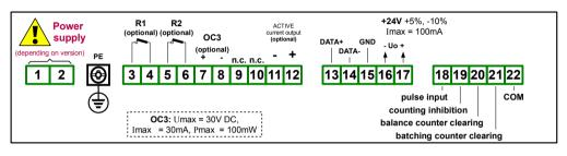
Figure 4.6. Terminals description (two relay, one OC-type and active current outputs)
