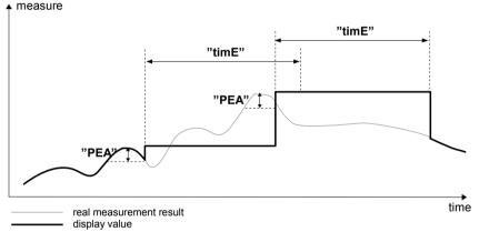
Figure 6.2. Process of peaks detection
