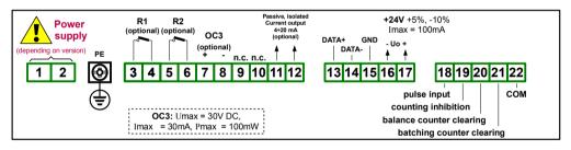
Figure 4.7. Terminals description (two relay, one OC-type and passive current outputs)
