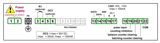
Figure 4.5. Terminals description (one relay and one OC-type output)
