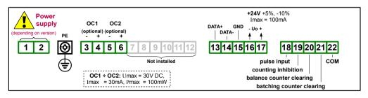
Figure 4.4. Terminals description (two OC-type outputs)
