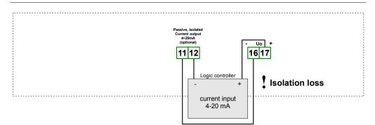
Figure 4.18. Example of passive current outputs connection (for device with passive current output only)
