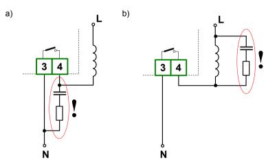
Figure 4.12. Examples of suppression circuit connection: a) to relay terminals; b) to the inductive load
