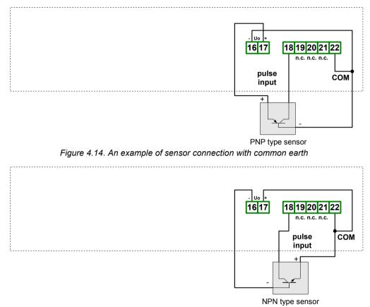
Figure 4.15. An example of sensor connection with common plus
