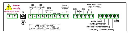
Figure 4.8. Terminals description (two relay, one OC-type and active voltage outputs)
