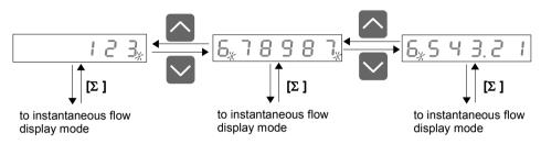
Figure 6.1. Switching between digits (screens) of total flow result.
