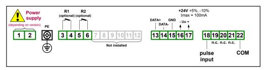
Figure 4.3. Terminals description (tow relay outputs)
