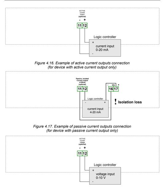
Figure 4.18. Example of active voltage outputs connection (for device with active voltage output only)
