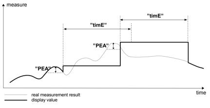
Figure 6.1. Process of peaks detection
