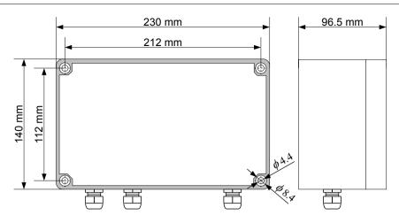
Figure 4.1. Device and assembly dimensions of the case
