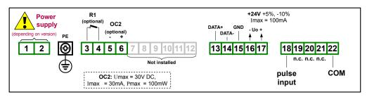
Figure 4.5. Terminals description (one relay and one OC-type output)
