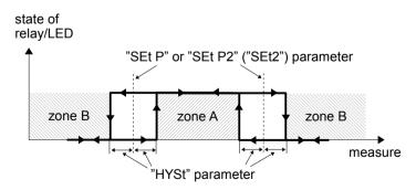
Figure 6.3. Two threshold control of the relay/LED outputs
