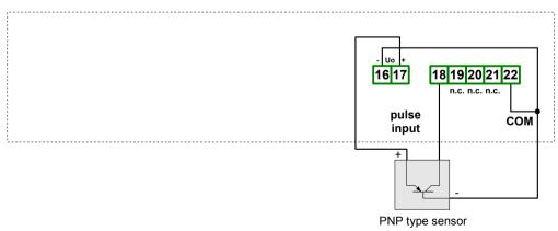
Figure 4.13. An example of sensor connection with common earth
