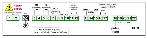
Figure 4.8. Terminals description (two relay, one OC-type and one passive voltage outputs)
