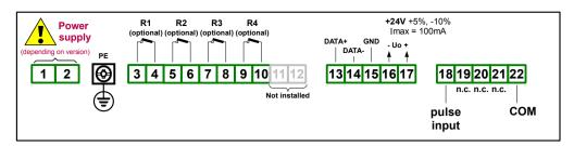
Figure 4.9. Terminals description (four relay outputs)
