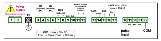
Figure 4.7. Terminals description (two relay, one OC-type and one passive current outputs)
