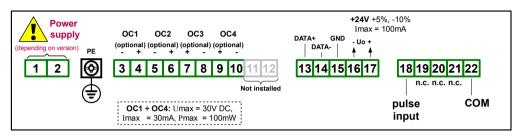
Figure 4.10. Terminals description (four OC-type outputs)
