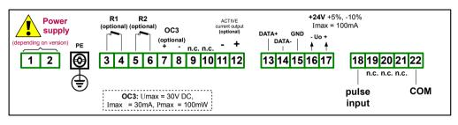
Figure 4.6. Terminals description (two relay, one OC-type and one active current outputs)
