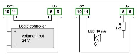
Figure 4.17. Example of OC-type outputs connection
