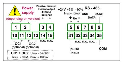
Figure 4.12. Terminals description (OC-type and passive current outputs)
