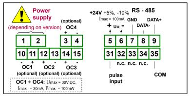
Figure 4.7. Terminals description (OC-type outputs)
