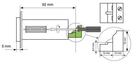
Figure 4.3. Installing of brackets, and dimensions of connectors.
