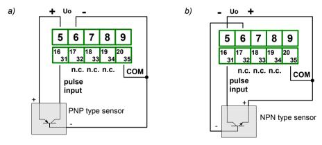
Rys. 4.16. An example of sensor connection: a) with common earth, b) with common plus
