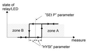
Figure 6.2. One threshold control of the relay/LED outputs
