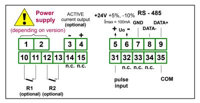
Figure 4.8. Terminals description (relay and active current outputs)
