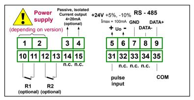
Figure 4.9. Terminals description (relay and passive current outputs)
