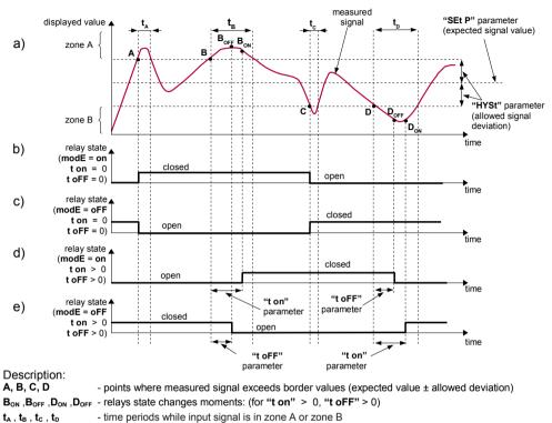
Figure 6.4. Principle of LED/relay output operation for one threshold mode
