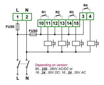
Figure 4.14. Connection of power supply and relays
