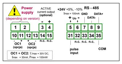
Figure 4.11. Terminals description (OC-type and active current outputs)
