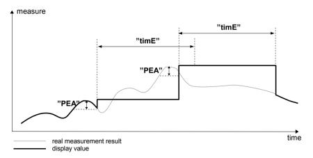
Figure 6.1. Process of peaks detection
