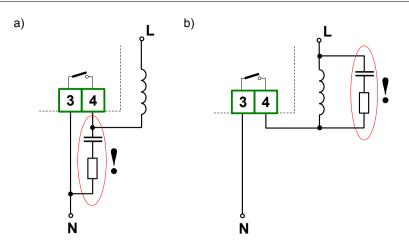
Figure 4.15. Examples of suppression circuit connection: a) to relay terminals; b) to the inductive load
