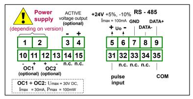
Figure 4.13. Terminals description (OC-type and active voltage outputs)
