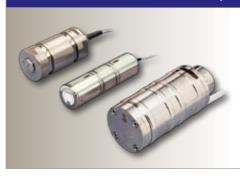
Vishay Systems offers a unique series of load beams for use as axles, pins, and shafts. These cells replace "dead" shafts in bogies, pulleys, and coupling devices, thereby providing live force measurement for crane scales, aircraft/ship wheel bogies, push-pull systems, and other onboard devices.
