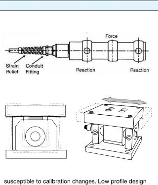
susceptible to calibration changes. Low profile design and symmetrical mounting bolt patterns make KDH modules easy to install on new or existing structures and vessels.
