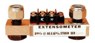
With extensometers installed, the mill posts become an active part of the measuring system. The entire mill housing with the attached extensometer can be considered a "load cell".
