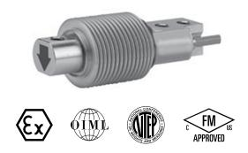
The low profile, high accuracy and sealing makes this load cell highly suitable for applications such as low profile platforms, weighing and packing machines, conversion of mechanical and a variety of other applications where sealed cells are required. For hazardous environments this load cell is available with EEx ia IIC T6 level of approval as an option.
