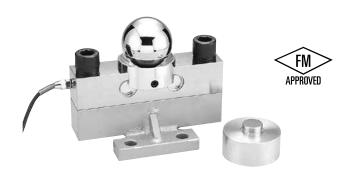
The Model MDB is constructed of alloy steel and is fully potted and sealed with special chemical compounds to IP67, providing excellent protection against water and moisture attack. With hermetic sealing, the MDB is rated for IP68 providing excellent protection against corrosive and wash-down environments.
