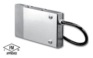
The stainless steel construction and IP67 sealing make this load cell ideal for very harsh environment applications. This load cell is specifically designed for use in corrosive and wet environments that are not appropriate for common aluminum load cells.
