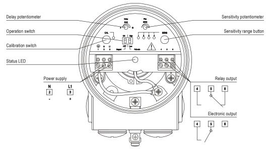
Wiring of relay and electronic output versions
