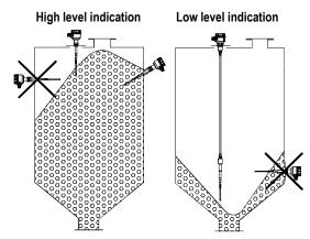
In case of powder level detection the device should be installed that the inclination of the side mounted probe should be greater than the angle of repose (or, in case of high level detection vertically), to prevent powder deposition on the probe that might cause false switching. Also avoid mounting the unit near to recess or near to any surface that facilitate build-up forming.
