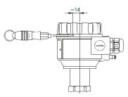
This case the status LED will blink blue during the calibration. All the other configuration settings (Sensitivity range selection, Sensitivity fine adjustment, Delay adjustment, Fail-safe operation mode selection and switching the Magnetic Calibration switch to <u>ON state</u>) should be carried out outside the hazardous environment (e.g. in the control room) before mounting the instrument.
