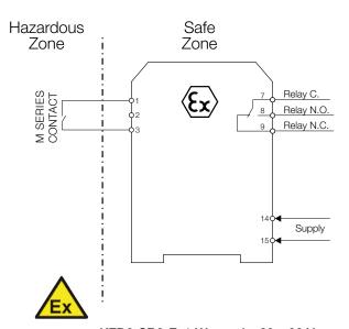
KFD2-SR2-Ex1.W supply:  $20...30 V_{DC}$ KFA6-SR2-Ex1.W supply: 207...253 V<sub>AC</sub>
