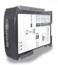
the MODBUS protocol and able to control more complex systems. The WT2 also features an optional Ethernet connection, which comes with a 128-byte in/out buffer for high-speed PC connections. The Ethernet cable can be augmented with the PROFINET protocol, which enables full integration into systems with that protocol.
