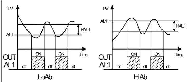
**LodE** = DEVIATION LOW ALARM: The alarm is activated when the process value goes below the value [SP + AL1] and will be deactivated when it goes above the value [SP + AL1 + HAL1].
