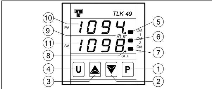
**1 - Key P** : This is used to access the programming parameters and to confirm selection.
