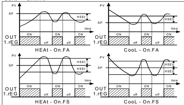
The control works in the following way : in the case of reverse action, or heating ("Func"=HEAt), it deactivates the output, when the process value reaches [SP + HSEt] in case of symmetrical hysteresis, or [SP] in case of asymmetrical hysteresis and is then activated again when the process value goes below value [SP - HSEt].
