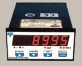
Batching system weighing indicator provides digital or isolated analog output signal for tank/bin/hopper weighing systems. An isolated 0–10 V or 4–20 mA analog output provides factory floor communication for a data logger, remote panel meter, or PLC input. High level serial communication is available in RS232, or RS485 format with Modbus RTU or Profibus protocol. Up to 32 transmitters can be connected point-to-point.
