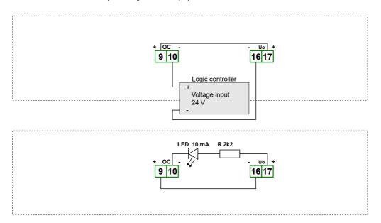
Figure 4.16. Example of OC-type outputs connection
