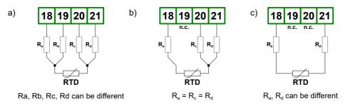
Figure 4.13. Connection of RTD sensors:
