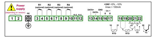
Figure 4.5. Terminals description (four relay outputs)
