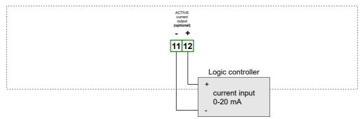
Figure 4.17. Example of active current outputs connection (for device with active current output only)
