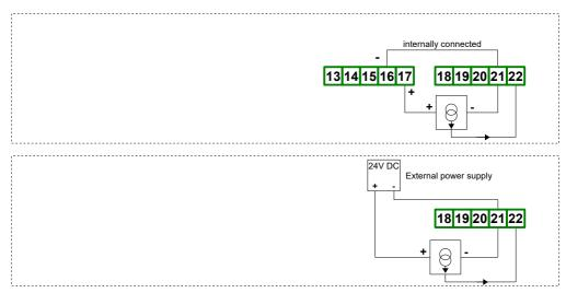
Figure 4.11. Connection of 3-wire current converters
