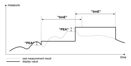
Figure 6.4. Process of peaks detection
