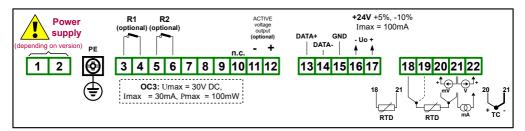
Figure 4.9. Terminals description (two relay and active voltage outputs)
