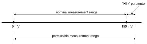
Figure 6.2. Definitions of measurement ranges in mode 0 ÷ 150mV
