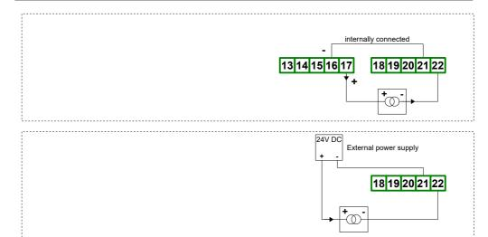
Figure 4.10. Connection of 2-wire current converters
