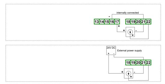
Figure 4.12. Connection of voltage converters
