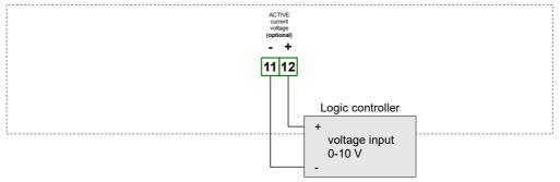
Figure 4.19. Example of active voltage outputs connection (for device with active voltage output only)
