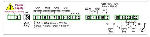
Figure 4.6. Terminals description (four OC-type outputs)
