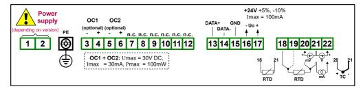
Figure 4.4. Terminals description (two OC-type outputs)
