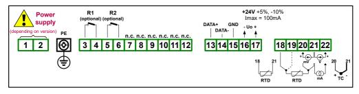
Figure 4.3. Terminals description (two relay outputs)
