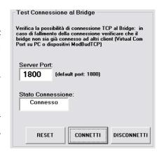
WT 2/Ethernet can accept and maintain only one connection; before the test of the connection make sure that other client devices in the network are not associated with WT 2/Ethernet.
