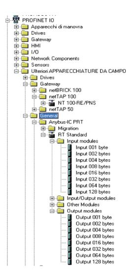
3. Enter inputs and outputs to 128 bytes and associate desired address, define the name of the object eg. WT 2, it will serve for naming the network.
