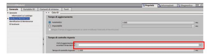
4. Through assigns name to the device, select the module to be parameterized, define in the configuration of WT 2 the IP address, see PARAMETERS SERIAL OUTPUT. Assign to the module the IP configuration and device name; The device name must be the same as defined in the hardware configuration DEVICE NAME. If the IP address and the NAME UNIT are not defined and equal, the module is not recognized in the profinet network.
