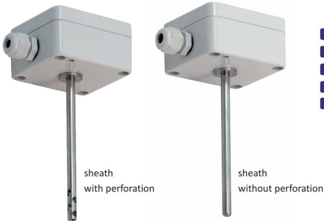
Resistance thermometers **SCR500** are designed for ambient temperature measurement. There is a possibility of assembling a programmable temperature transmitter with a 4...20 mA output signal into the housing. The protection tube with perforation allows for quick and precise temperature measurement, thanks to direct contact of thermometric resistor with ambient temperature.
